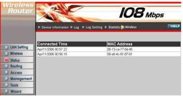
**Connected Time:** Displays how long the wireless device has been connected to the LAN via the router.
